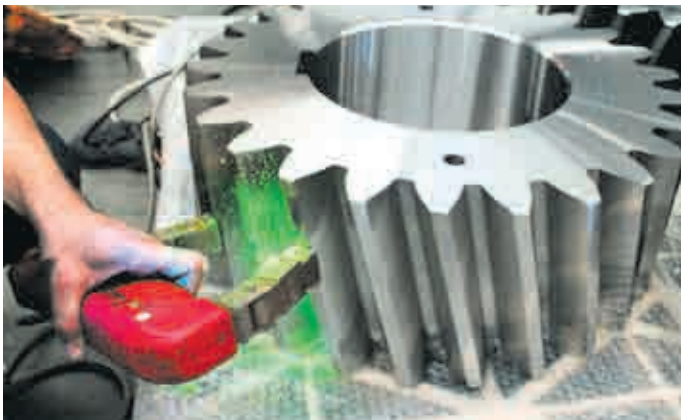
Manyetik Kontrol / Magnetic Particle Inspection
